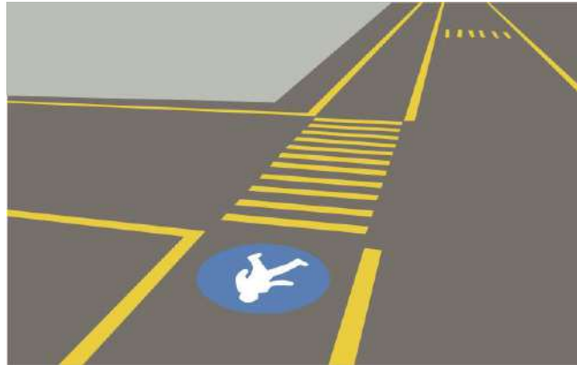
Fig.: 5.3 – Yellow Demarcation for Pedestrian Pathway
