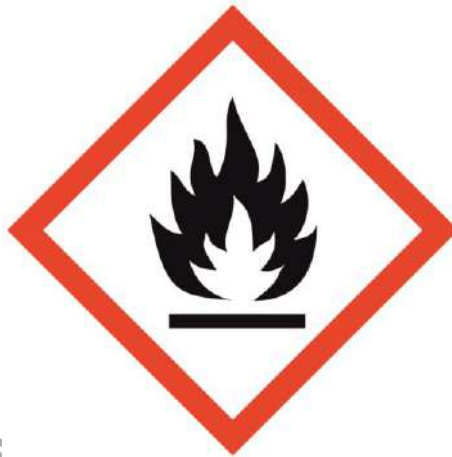
Fig.: 5.17 - Flammable substance Sign
